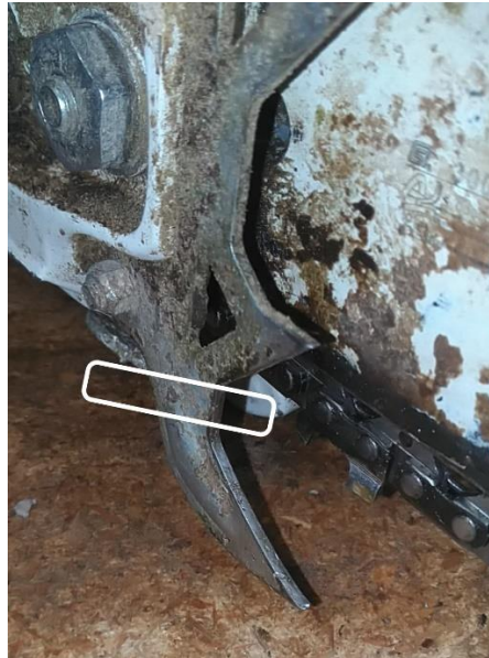
Figure 11 - Close-Up of Bent OEM Felling Spike
