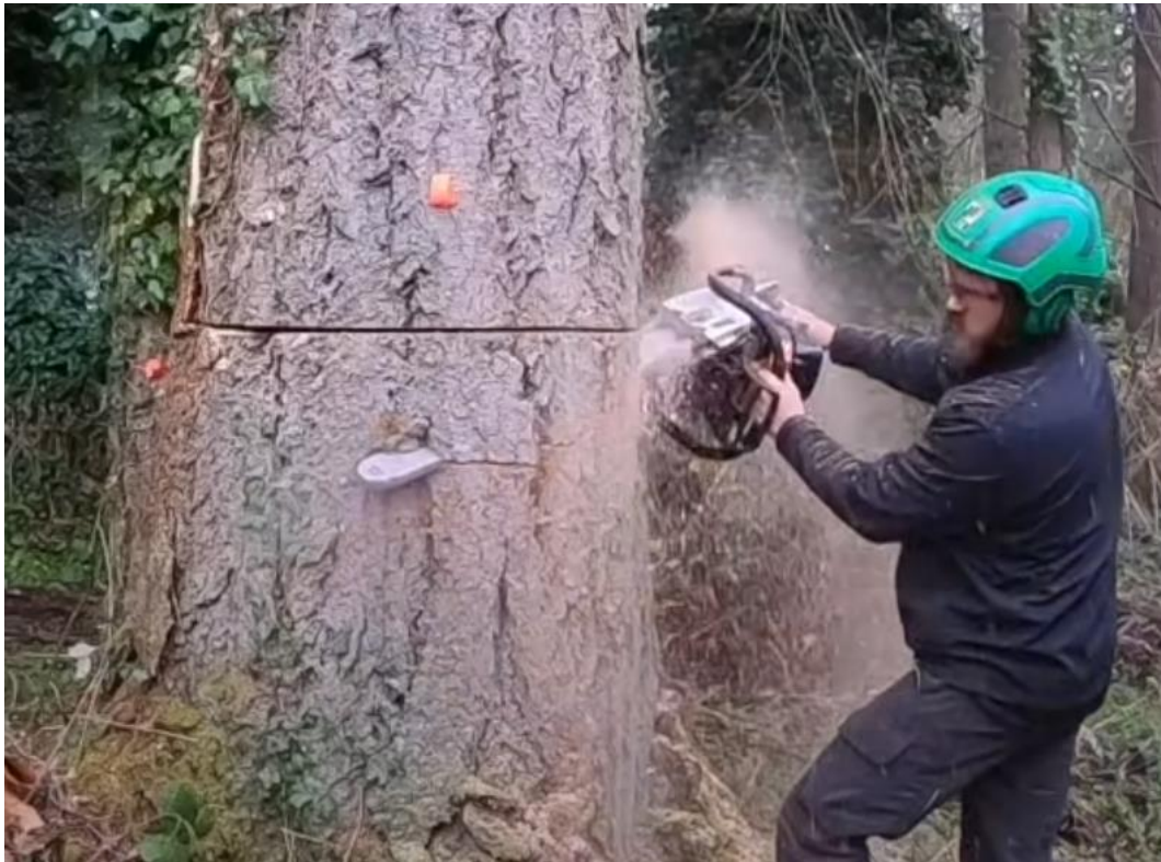
Figure 4 – Professional Employing Chainsaw Felling Dogs to Place Cut #2 in a Humbolt Notch Felling Spikes are in Active Use for this Situation (Guilty of Treason Image) Operator Pushes Lightly Toward the Tree with his Left Hand While his Right Hand Pulls Back Cuts #1 and #2 meet on Opposite Sides of the Tree for the Notch
