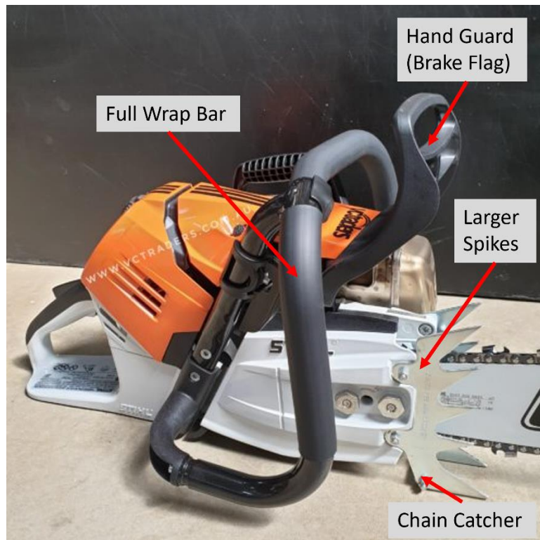
Figure 2 - 500i-R with Full Wrap Handle, Larger Cover, and Larger Felling Dogs/Spikes
